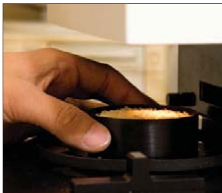
NIRS – Researchers are developing a system based on near infrared spectrometry (NIRS) to provide data on multiple rice quality traits in seconds compared to hours using current methods.
